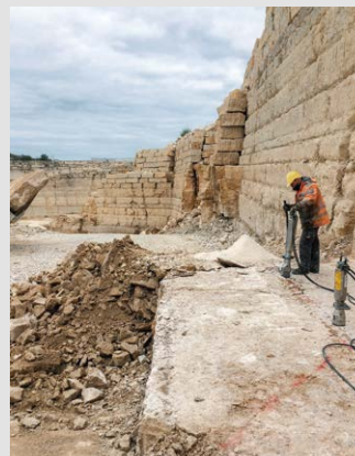
Block quarrying in the natural stone industry
